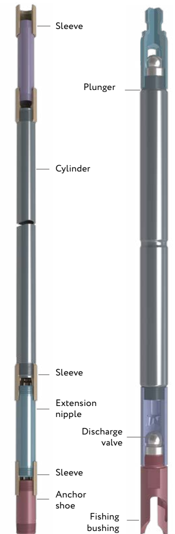
Scheme of a tubing pump THM with mechanical fastening of a suction valve according to API
