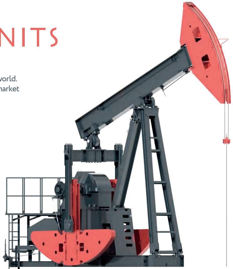
While we manufacture pumping units in full compliance with API Specification 11E, there is a significant benefit of GOST standard surface units – the application of the Novikov gearing reducer instead of the involute gearing, as required by API.
